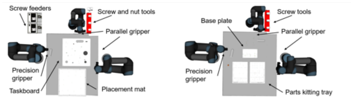
Figure 6. Top view of the scene layout in the taskboard (left) and assembly (right) tasks.
