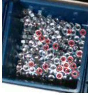
Figure 14. Result of searching for the graspable hole in M4 nuts, based on 2D contour detection method.
