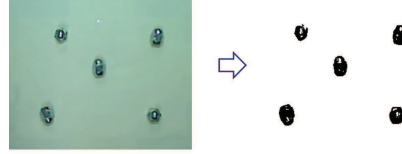
Fig. 2. RGB image (left) and its binarized image (right) of a few shiny objects placed on a table
