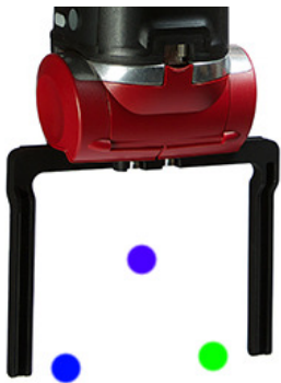
Fig. 3: Robot end effector encoded as 3 points in space. Each point is represented by its x , y , z component.
