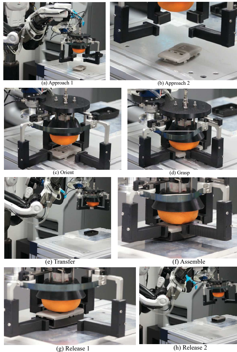
Figure 16. Snapshot of assembly experiment of Parts 1 and 2
